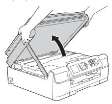
b Connect the USB cable to the USB port marked with a + symbol. You will find the USB port inside the machine, as shown in the callout below.
